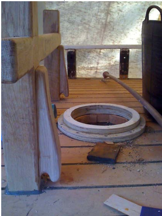
Fife rail and mast aperture
