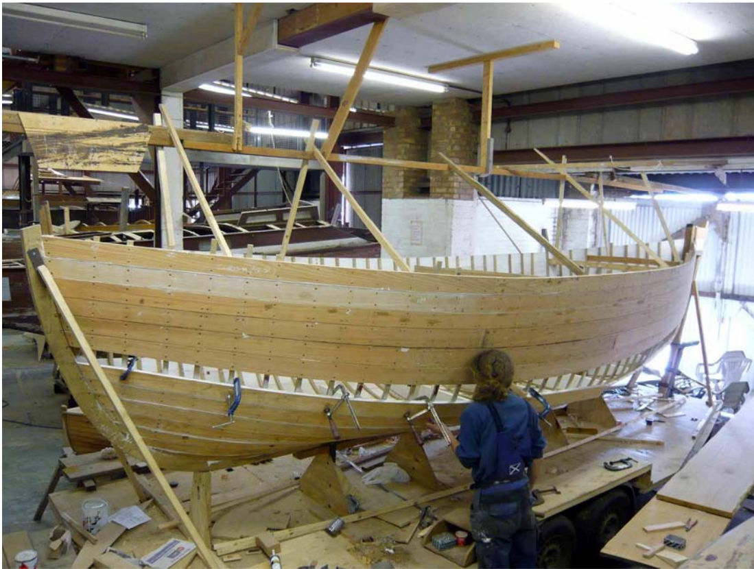
Replica Caird – planking almost complete
